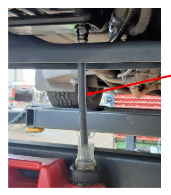
Example: How to use the oil drain valve
